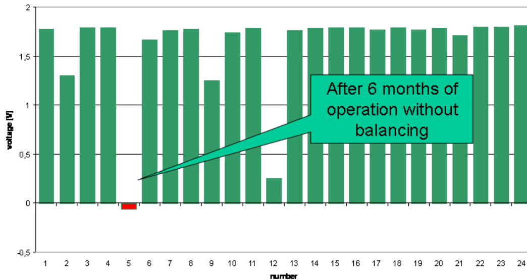
Figure 28: Individual cell voltage after 6 month of operation without balancing.
