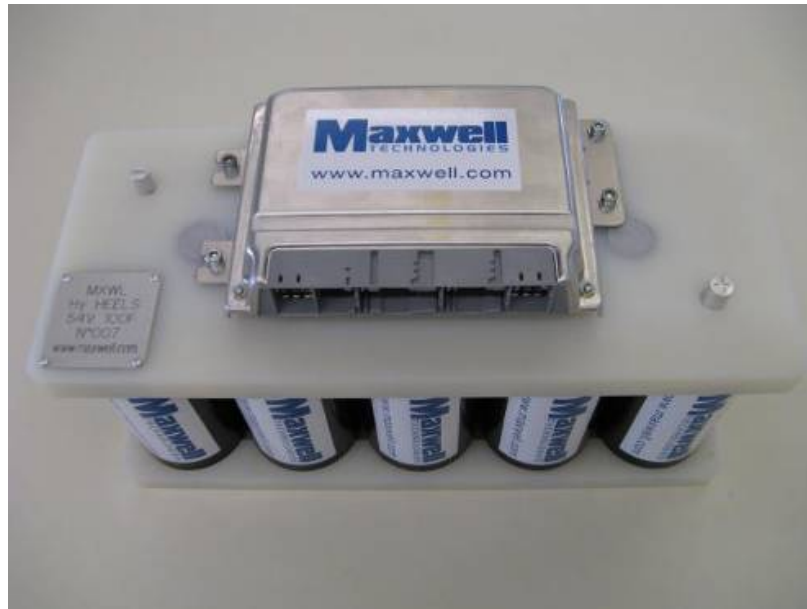
Figure 3: HyHEELS module 54V 100F in final version, including the controller
