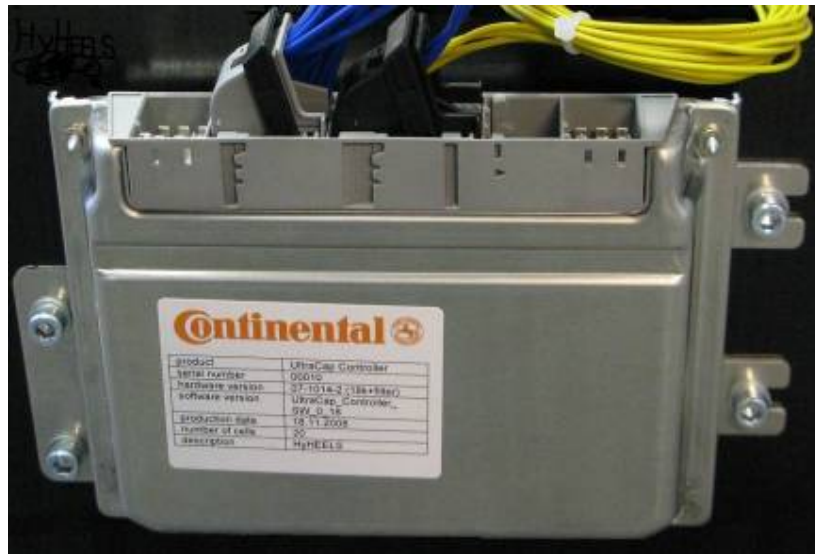
Figure 51: Picture of fully assembled UltraCap controller
