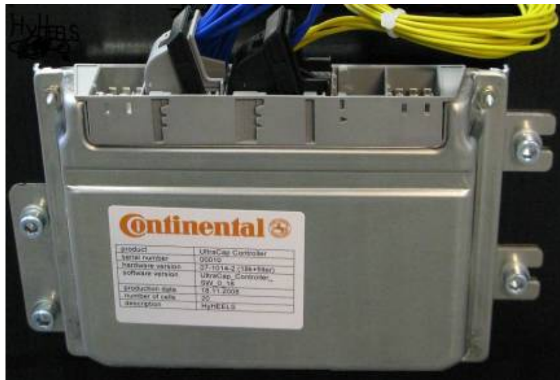
Figure 7: Picture of fully assembled UltraCap controller
